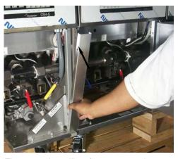
Figure 8. Installing front connecting post on connected fryer sections.
